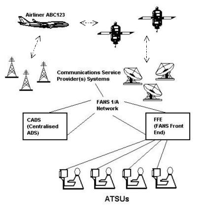
2.3.2 ATS Facilities Notification (AFN) Logons received from aircraft provide each ATSU with the information required to correctly route CPDLC messages between themselves and that aircraft.
